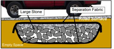
SIDE VIEW SCHEMATIC OF A FRENCH MATTRESS (SOURCE: PENN STATE CENTER FOR DIRT AND GRAVEL ROAD STUDIES)
