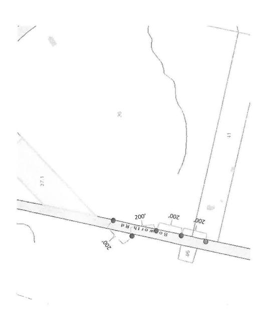
Extend 4 fully owned poles in a northeast direction for 800' to fed 42 Bosworth Rd, Sandisfield wo#11702443 Fwo#80511691 this new customer
